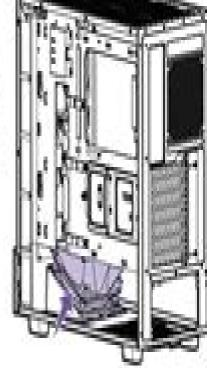
From the trust size of the shrout, lift the air duct and remove it from the case.
