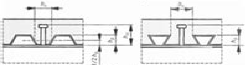
3. : Beam with profiled steel sheeting transverse to the beam
