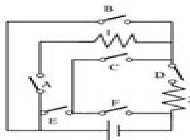
*In the diagram at the left you will need to decide which switches to close to allow different resistors to have current flowing thru them. This is like maze games—just follow the path. But here are the rules: 1) you must start at the + side of the battery (big side) and get back to the - side; 2) you can't go backwards along the same line (since current only flows from high V to low V); 3) you can't make a short-circuit (make a circuit without a resistor in it).*
