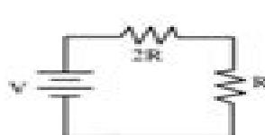
3. The new symbol you see in the diagram at the left is a multicell battery (like a 9V), which is made up of a number of smaller single cell batteries (like a 1.5V). Let's say its total voltage is  $V$ .
