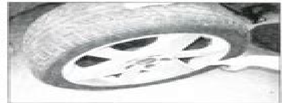
6 If the tyre is flat make sure that the vehicle is raised sufficiently to allow the spare wheel to be fitted. Remove the bolts and lift the wheel from the vehicle. Place it beneath the sill in place of the spare as a precaution against the jack failing.
