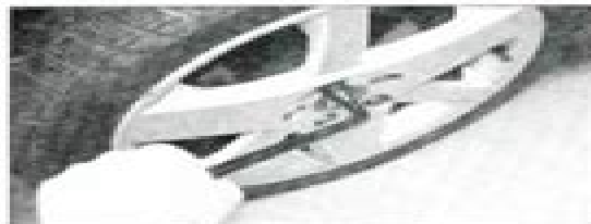
4 Before you raise the car, loosen each wheel bolt by half a turn only.
