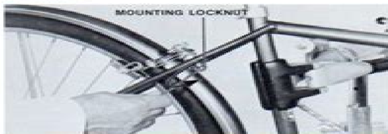
FIGURE 2—LOOSENING MOUNTING LOCKNUT
