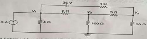
B) State Superposition theorem and Find the current in the I  $\Omega$  resistors
