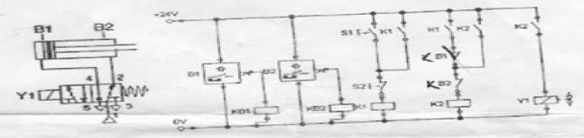
Q3 Design a circuit in which a double acting cylinder is used to press together the glued components. Upon operation of a push button, the clamping cylinder extends. Once the fully advanced position is reached, the cylinder is to remain for a time of T=6 seconds and then immediately retract to the initial. The cylinder retraction is to be adjustable. A new start cycle is only possible after the cylinder has fully retracted.
