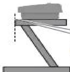
Align the front of the frame with the front of the stand.
