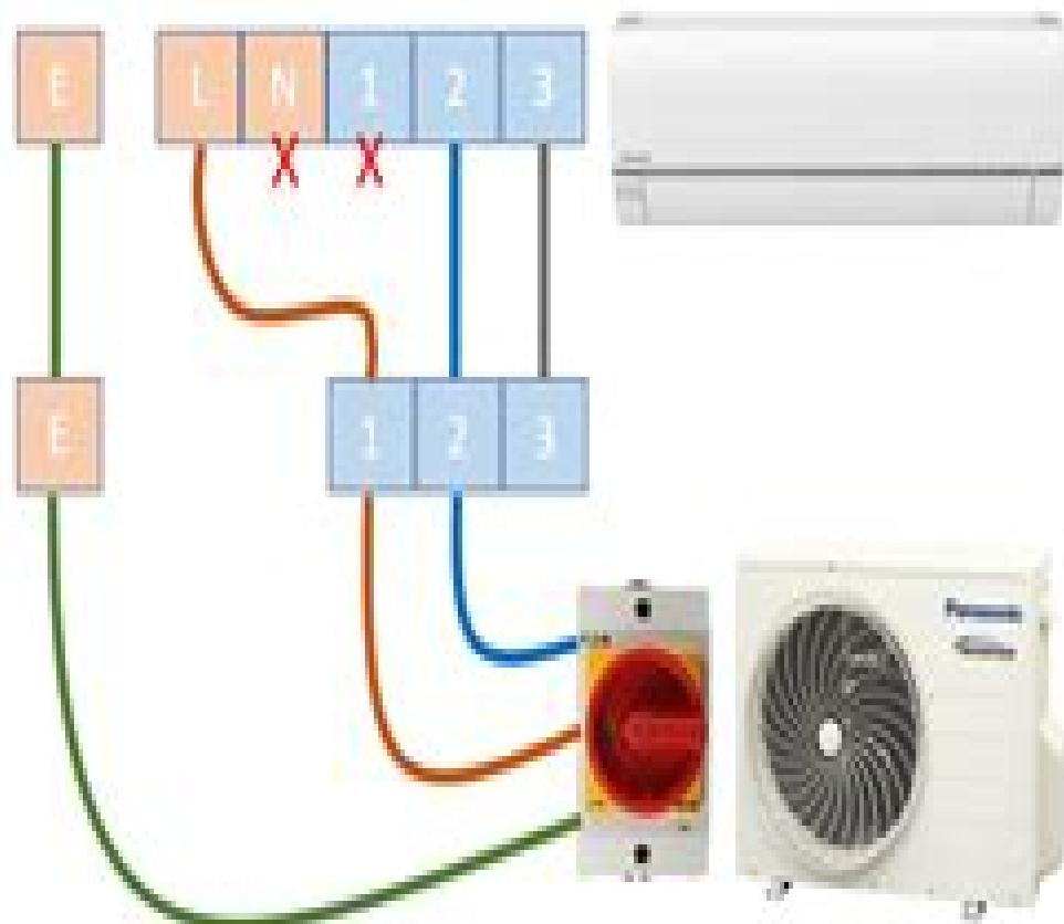
Applies to RE, TE, FE, FZ, TZ, Z, XZ models. Note where the LIVE wires to for each option
