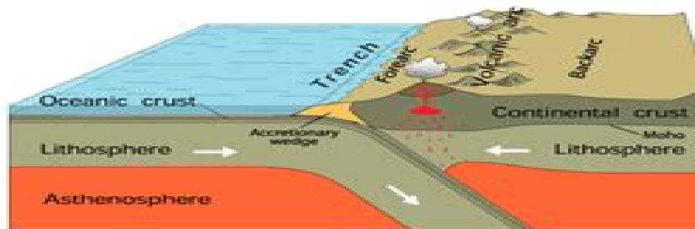
Figure 1. A subduction zone where an oceanic plate slides beneath a continental plate. [USGS]
