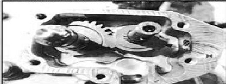
18. Install the detent pawl (I) onto the shift shaft. Install the detent star (J). Install a new O-ring onto the shift shaft. Apply a small amount of grease onto the O-rings and end of the shift drum.
