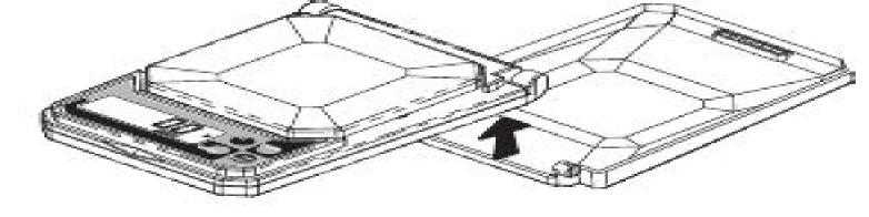
Re-attach the cover by pushing scale down onto the lid and snapping the hinge back in place.
