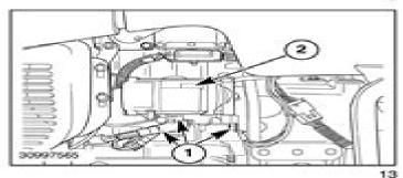
If equipped with FWD, remove the roll pins, 1, from the front and rear of the FWD driveshaft, 2, and remove the driveshaft from the tractor.
