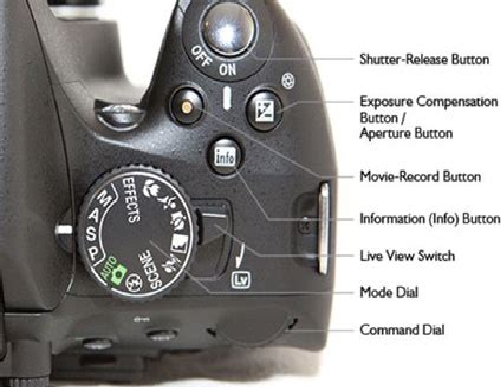
Figure 2 - Controls on the top of the D5100
