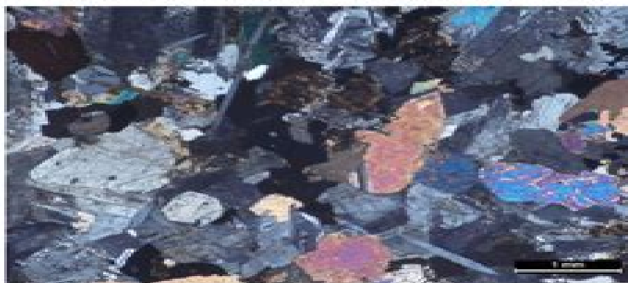
Figure 4.1 – Thin section view with crossed polarizers showing interlocking crystals of pyroxene (colorful grains), biotite (dark brown) and plagioclase feldspar (white to black striped grains) in a coarse-grained igneous rock. See also Figure 2.5.
