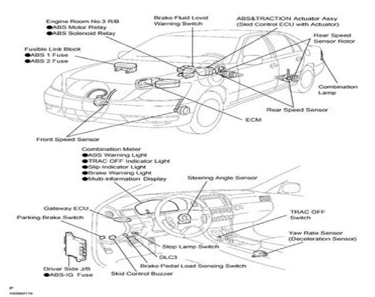
Fig. 1: Identifying ABS With EBD & BA & TRAC & VSC System Components Location Courtesy of TOYOTA MOTOR SALES, U.S.A., INC.
