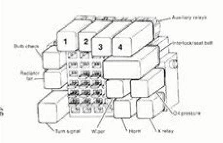
Shortly after the start of 1983 model production, relay locations will be changed. The oil pressure relay will be relocated to the fuse panel (it was taped to the instrument cluster harness) and the fuel pump relay will be clipped to the top of the fuse panel. vdubspeed was here.
