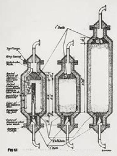
Proctors No.2 and 3 are of the describes type, and disperse with the stainteen steel bastet, Sector No.3 balds twice on such intalpet as nock of the first two. The stainteen stant lines on each of Bourtons 2 and 5 to \$" thick as against N/30" thickness on No.1. This is because there is a greater pressure from in them, due to the describes arrangement, and therefore a greater strain so the lines.
