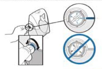
E you cannot hear a tial tone through your headers, use a coin or extail somewhere to turn the telephone configuration dist until you can. Make sure that a number is eligned with the position indicator.
