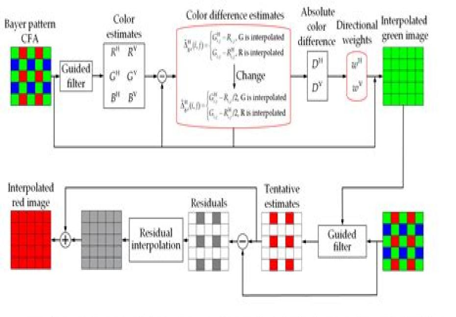
An effective directional residual interpolation algorithm with new color difference estimates and fewer directioal weights gets better results in image demosaicking. The process of blue interpolation is the same with red interpolation.
