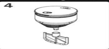
Attach the mixing rod to the motor part.
