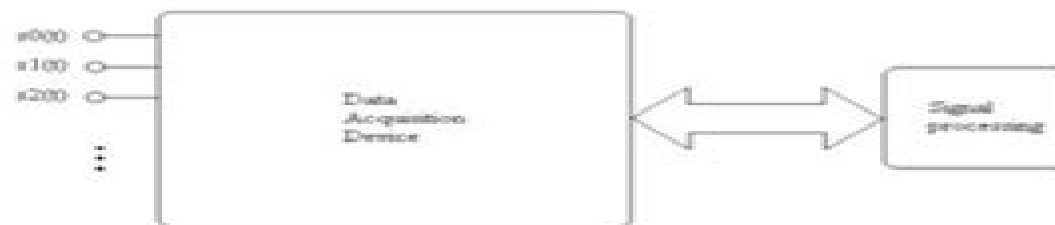
Fig. 1 A rough structure of the PC based oscilloscope
