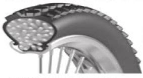
The air particles inside the tire hit the walls of the tire with a force. This force produces a pressure inside the tire. The pressure keeps the tire inflated.
