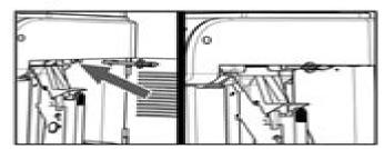
Warning! Disabling the safety microswitch entails a danger for the operator to come into contact with the moving parts of the appliance. Enable the safety device again right after completing the adjustment.
