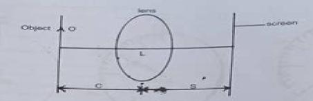
The diagram above shows an illuminated object O placed at a distance C in front of a converging lens L and its image produced on a screen R which is placed behind the lens.
