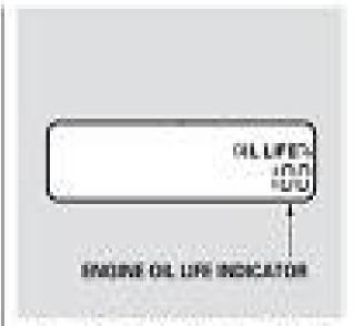
Press the TRIP betton for about 5 seconds. The maintenance items code(s) will disappear, and the engine oil life will reset to "100."
