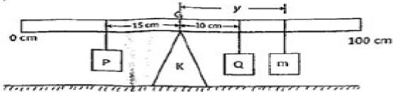
You are provided with a metre rule, two loads, P and Q, a knife edge, K, a set of masses, m and a piece of string.
