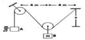
The system of masses A and 8 shown in the figure is released from rest with x = 0. If the velocity of mass B and x = 3m is 'v' and its maximum displacement is x ,, then choose the correct option
