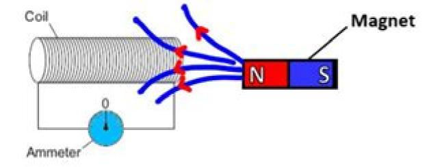
The ammeter has a centre zero scale, so that values of current going in eithrough
