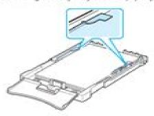
NOTE: If you want to change the size of the paper in the tray, refer to "Changing the Size of the Paper in the Tray" on page 2.5. 7 Squeeze the paper length guide and slide in it until it lightly touches the end of the paper stack.
