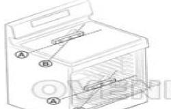
Use a level to check your adjustments. Place the level diagonally on the oven rack or surface cooktop, and confirm the range is level in the two directions shown below.
