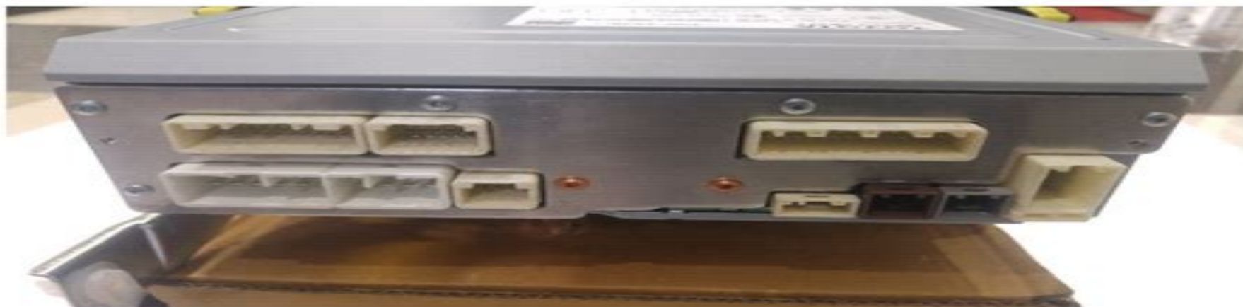
16 pin (10+6) Toyota Head Unit proprietary connector
