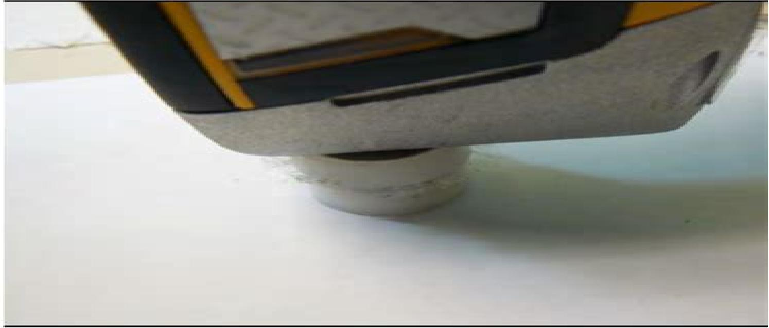
2. Place the analyzer so the sample is covered by the analysis window.
