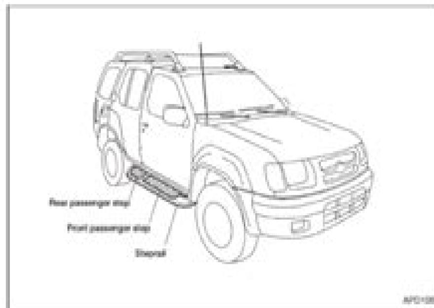
The step rail has a front and rear step for assisting passengers to get into and out of the vehicle.
