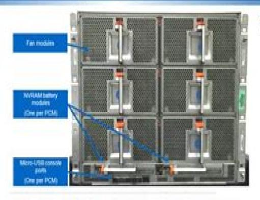
PCM: Processor Controller Module
