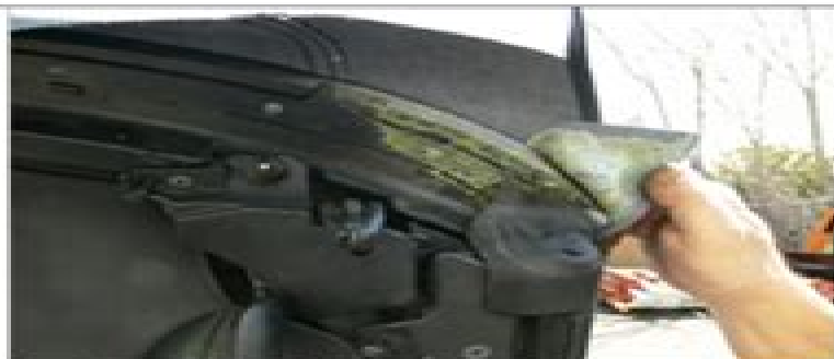
Step 25: FRONT CORNER FLAPS. Apply contact cement by spray to top front corner flaps and frame.
