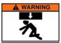
To avoid crushing and related injuries: MEVER work on, under or around a load supported only by a jack. ALWAYS use adequately rated jack stands.
