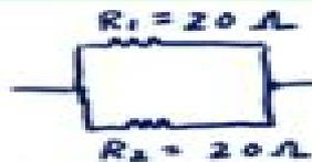
$$R_{1,2} = \frac{1}{\frac{1}{R_1} + \frac{1}{R_2}} = \frac{1}{\frac{1}{20\Omega} + \frac{1}{20\Omega}} = \frac{1}{\frac{2}{20\Omega}}$$
