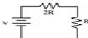
3. The new symbol you see in the diagram at the left is a multicell battery (like a 9V), which is made up of a number of smaller single cell batteries (like a 1.5V). Let's say its total voltage is V.
