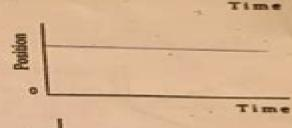
The object moves with a steady (constant) velocity toward the origin for 5 seconds and then stands still for 5 seconds.
