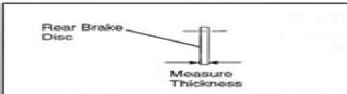
**Brake Disc Thickness**
