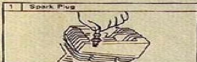
Ground the spark plug to the cylinder head and kick the starter.
