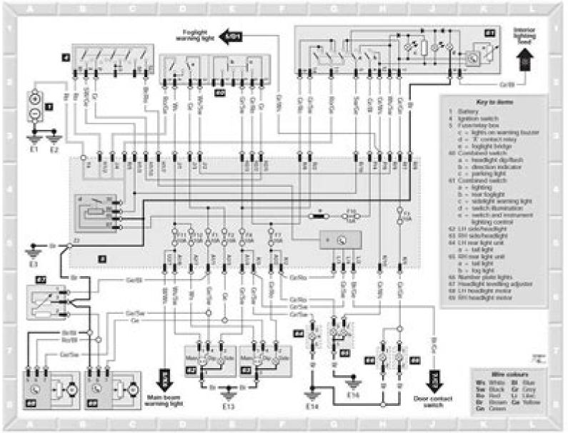
Diagram 6 : Side, tail, number plate, head and foglights, headlight levelling - models up to 1998
