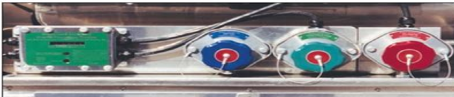
Scully truck mounted control monitor and sockets
