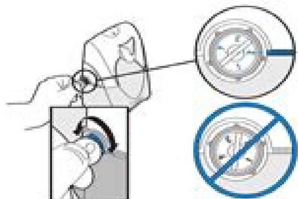
If you cannot hear a dial tone through your headset, use a coin or small screwdriver to turn the telephone configuration dial until you can. **Make sure that a number is aligned with the position indicator.**
